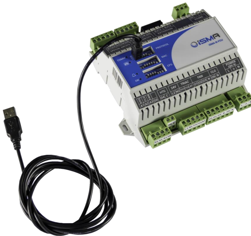
Figure 46. Direct connection to iSMA-B-FCU controller
